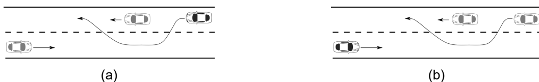
Figure A2.13: Overtaking with oncoming object (a) active or (b) passive scenarios.
