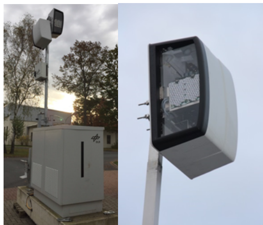
Figure 4.2: AIM Mobile Unit and sensor head.
