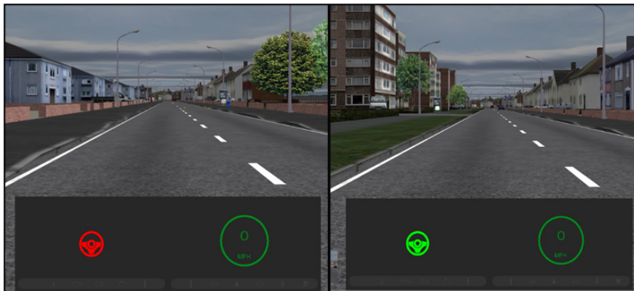
Figure 5.1: An example of the in-vehicle HMI with the automation status symbol (Left: automation not engaged, Right: automation engaged) and the vehicle speed (mph).
