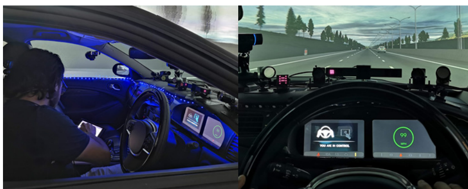
Figure 5.2: Example of the Lightband HMI during automated driving (left), and the placement of the automation status symbol and vehicle speed in the dashboard display (right). In both figures, the Driver Monitoring System is located on the dashboard above the steering wheel.
