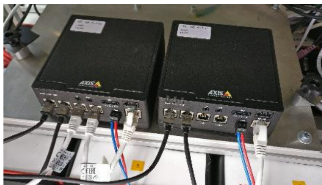
Figure 2.1: Setup of two Axis F44 base units to collect USB camera video feeds.
