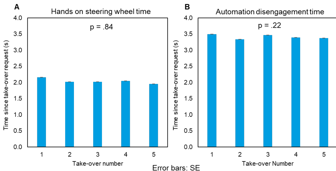
Figure 10.6: Time taken from take-over request was issued to A) both hands on wheel, and B) automation disengagement, for each take-over. Error bars represent Standard Error.
