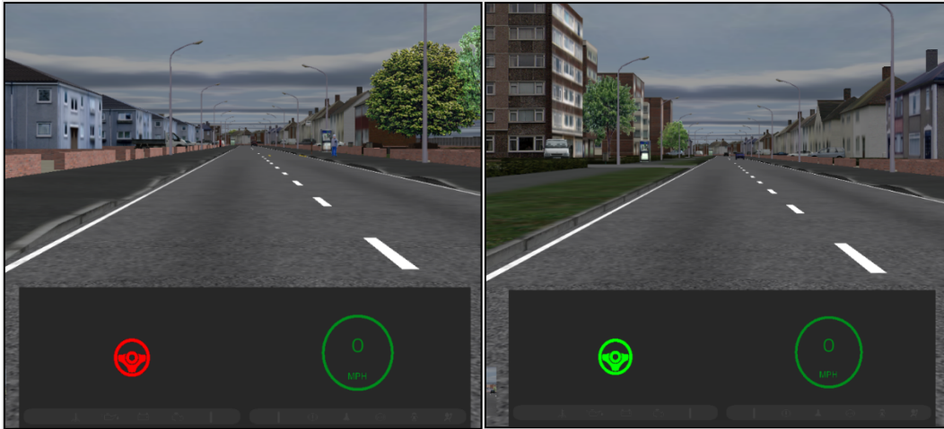
Figure 9.1: An example of the in-vehicle HMI with the automation status symbol (Left: Automation not engaged, Right: Automation engaged) and the vehicle speed (mph).
