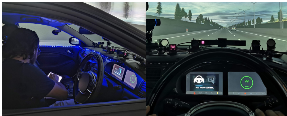
Figure 10.3: Example of the Lightband HMI during automated driving (left), and the placement of the automation status symbol and vehicle speed in the dashboard display (right). In both figures, the Driver Monitoring System is located above the on the dashboard above the steering wheel.
