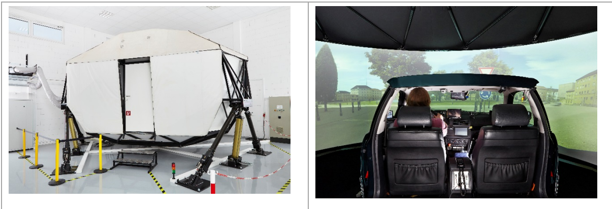
Figure 5.1: WIVW's motion-based driving simulator from the outside (left) and from the inside (right).
