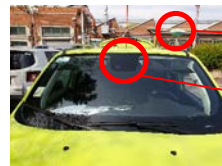
Antenna for DGPS
