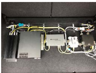
Trunk lid (eHMI ECU, PC, camera unit)
