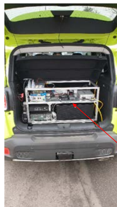
Trunk of CRF vehicle (including Lidar ECU, CCPU and E/E components)
